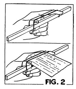
The elevator has its leading edge resting on the lower of the two frame blocks. 4 1/2" back from the nose. Attach in this position with two bands as shown.
