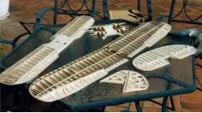
Wing and tail components. Note the use of balsa sheet cores on ailerons and tail assembly. This is a simple and strong means of construction.
