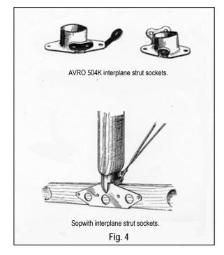
The incidence wires, together with the landing and flying wires, create sufficient up and down loads to maintain the struts in the sockets. The DH9A interplane strut is attached as per (Fig.5).
