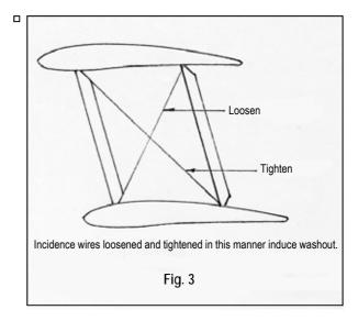
You can also alter the wing stagger which really induces internal stresses, remember the root of the wings are attached to the fuselage and centre section struts. These can be tilted forward or aft by adjusting their incidence wires, you may also have to alter the strut length to maintain the predetermined incidence. As you can see it's no wonder that this process required the dedicated attention of a trade person that's almost non-existent to-day— the Aircraft Rigger.
