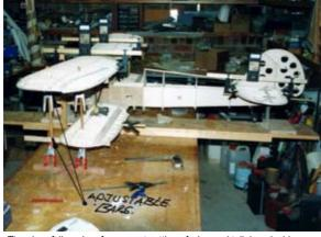
The aircraft jigged up for correct setting of wing and tailplane incidence. Barrie has invested heavily in Robart incidence meters.
