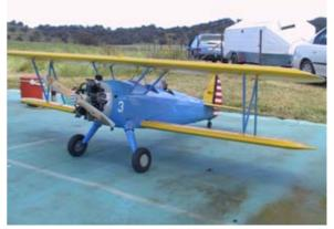
Clive Butler's 1/3 scale Stearman was very impressive as the 215cc, five cylinder, radial motor pulled the big airframe around the circuit. Probably the most realistic sound, apart from a jet turbine, that we have yet heard from a model engine.
