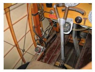
Finally, the engine suite is completed by a single ignition system with magneto on/off switch on the instrument panel and a blip button on the control column, which cuts out the ignition when depressed.
