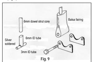
The horizontal tube is to take the mounting bolt and the vertical tube is to accommodate the 6mm dowel that is the structural core of the strut. Both on the Woodcock and the Ansaldo the core of the struts are encased in soft balsa shaped to represent the airfoiled strut. This soft balsa would then be a real bear to fill and finish by any normal method however I have a different approach which I pinched from Martin Fardell in England.
