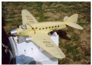
Steve Portelli's Savoia-Marchetti three engined airliner is very impressive in flight, but low wing models are at a disadvantage. The low engines tend to dig in on landing (wheels up!) damaging propellers and getting grit in the motors.
