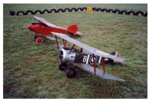
These two old timers flew around the circuit together at about the same speed. Andrew Smallridge's Camel is powered by a Laser 200 vee twin and weighs 6.5kg, compared with the Red Baron's Moki 180 powered Albatros at 9.5kg. The Camel proved agile enough to avoid the gunsights of its pursuer.
