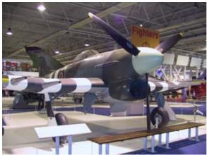
The Hawker Typhoon was designed as a high altitude interceptor but excelled as a ground attack aircraft with rockets and cannon.
