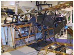
A Bristol Fighter with covering removed to show the construction.
