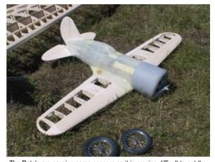
The Rata's are causing some concern as it is proving difficult to get the weight down for a reasonable wing loading. Fuselage and cowl is fibreglass. Wheels at the bottom of the picture are for the TB-3.
