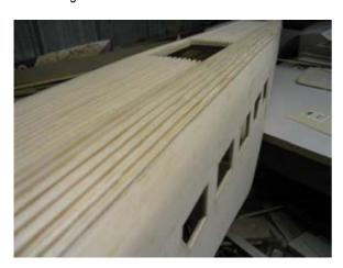
Once an area is corrugated it must be sanded down to a uniform height. I used a piece of brass tube of the desired diameter placed between the corrugations to sand down to. Next I made up a sanding block, a short length of 3/8" square hard wood with sandpaper
