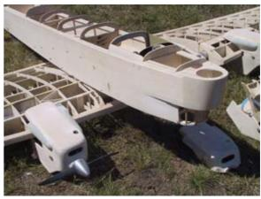
The TB-3 mother ship is conventional balsa/ply construction and will be covered with Solartex.
