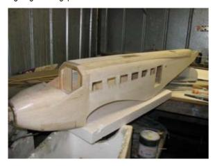
I started building last July and progress was rapid until I was confronted with the corrugations on the tail feathers and the fuselage. Having spent some time trying to work out the scale size of each corrugation I found that there were three different sizes. In an effort to keep the weight down I decided to make the corrugations out of strips of balsa.
