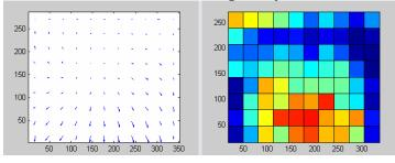
Fig. 3 Optic flow and divergence for forward translation
